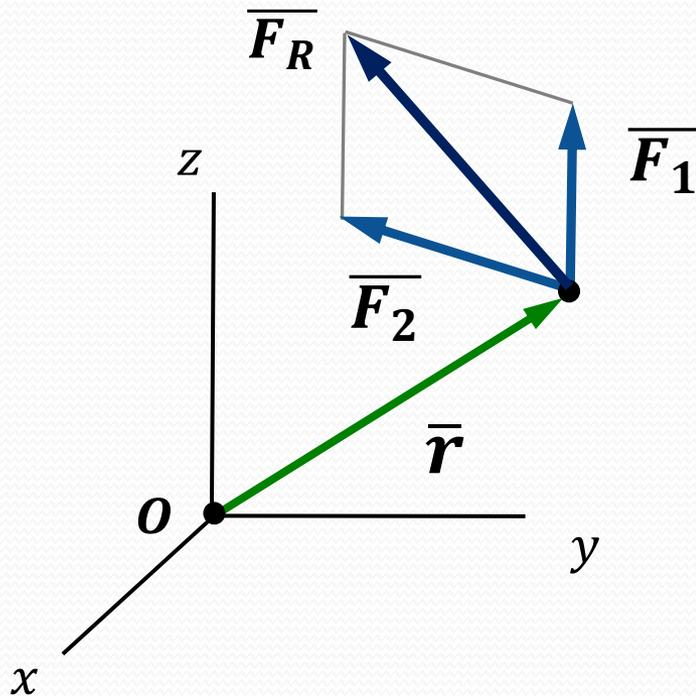
$$\overline{M}_{R_o} = \bar{r} \times \overline{F}_1 + \bar{r} \times \overline{F}_2$$
