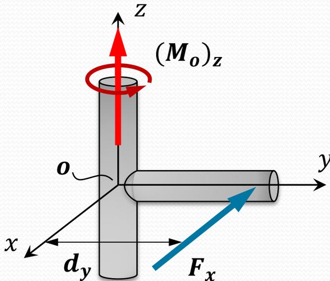
$$\begin{aligned}\bar{F}_x &\in XY \\ d_y &\perp \bar{F}_x \\ \Rightarrow (\bar{M}_o)_z &\perp XY\end{aligned}$$
