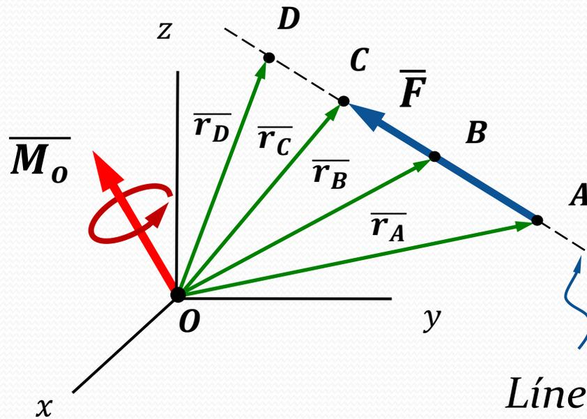
$$\begin{aligned}\vec{M}_o &= \vec{r}_A \times \vec{F} \\ \vec{M}_o &= \vec{r}_B \times \vec{F} \\ \vec{M}_o &= \vec{r}_C \times \vec{F} \\ \vec{M}_o &= \vec{r}_D \times \vec{F}\end{aligned}$$
