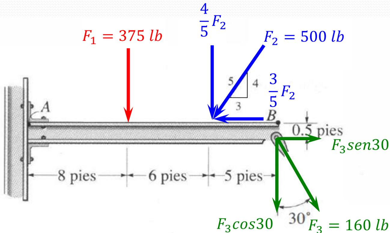
$$M_A = -(8)F_1 - (14)\frac{4}{5}F_2 + (0)\frac{3}{5}F_2 - (19)F_3 \cos 30^\circ + (0.5)F_3 \sin 30^\circ$$
