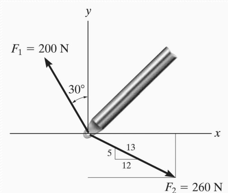
$$\begin{aligned}\overline{F}_1 &= (-200 \sin 30, 200 \cos 30) \\ &= (-100, 173.205) \text{ N}\end{aligned}$$
