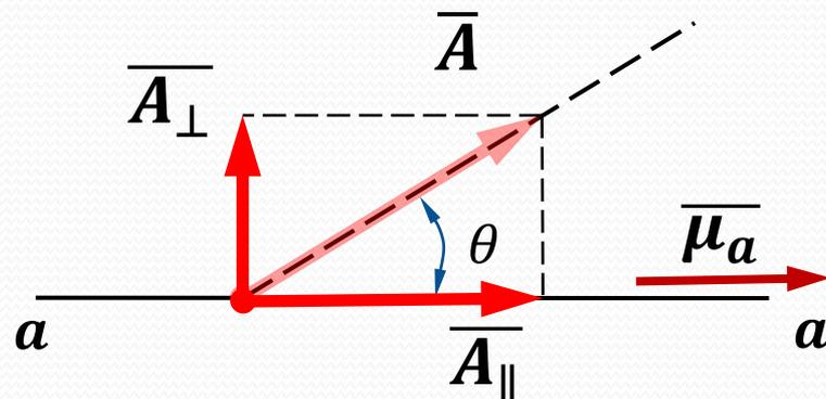
$$\bar{A}_{\parallel} = (\bar{A} \cdot \bar{\mu}_a) \cdot \bar{\mu}_a$$
