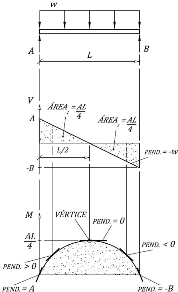
$$\begin{aligned} A_1 &= A \frac{L}{2} \frac{1}{2} = \frac{AL}{4} \\ A_2 &= -B \frac{L}{2} \frac{1}{2} = \frac{-BL}{4} \end{aligned}$$
