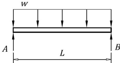
$$\begin{aligned} \Sigma F_y = 0: & \\ & A + B = wL \\ \Sigma M_A = 0: & \\ & BL = wL^2/2 \\ A = wL/2 & \quad \Delta \\ B = wL/2 & \quad \Delta \end{aligned}$$
