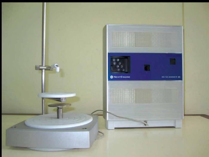
Escaner Láser: NextEngine Laser Scanner HD.
