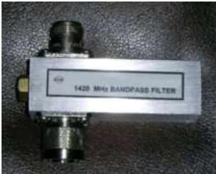
Low noise band-pass filter
