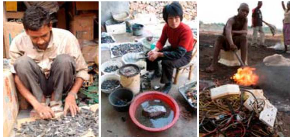
Figure 20. Recovery of valuable materials in e-waste by manual sorting, heating and burning of the electronic equipment, as carried out in many developing countries, e.g. India, China and Ghana. (Photos from left to right: © Prakash Hatvalne, Greenpeace, ©2006 Basel Action Network, and © Kate Davison, Greenpeace).
