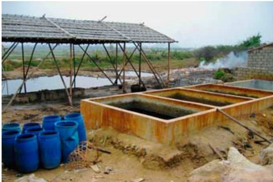
Figure 22. Site in Guiyu, China, where metals are extracted from PC-boards and other components, using strong acids such as aqua regia. (Photo: ©2008 Basel Action Network).
